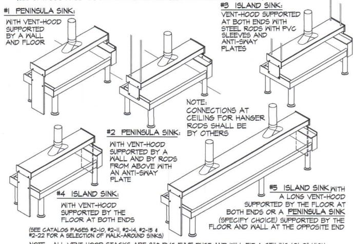
NOTE: ALL VENT-HOOD STACKS ARE 8" PVC FUME DUCT AND WILL FIT A CEILING 10'-0" HIGH
